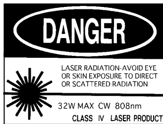
Label indicating that laser radiation exists inside.
