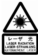
Label indication that laser radiation exists inside
